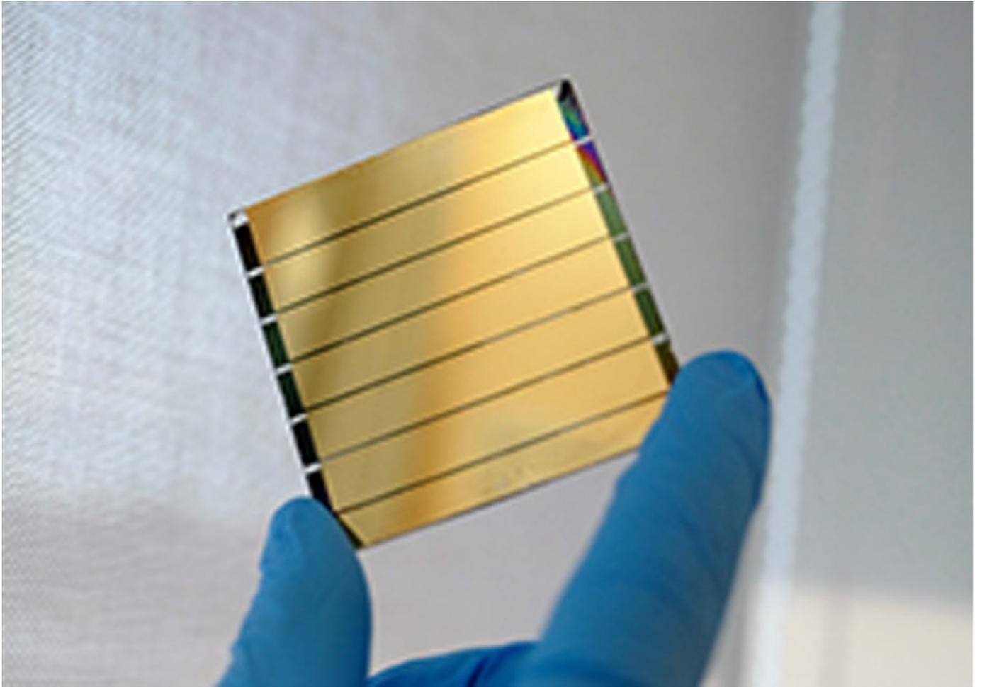
A team of researchers at the [Nanyang Technological University, Singapore \(NTU Singapore\)](#) has created a perovskite solar mini module that has recorded the highest power conversion efficiency of any perovskite-based device larger than 10 cm<sup>2</sup>.
