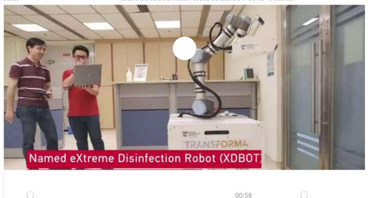
Researchers from @NTUsg have developed a disinfectant robot to aid cleaners in the fight against #COVID19. Able to move semi-autonomously, it can sanitise large surfaces quickly and operates for 4 hours continuously with its 8.5 litres tank and rechargeable batteries. Credit: NTU Singapore
