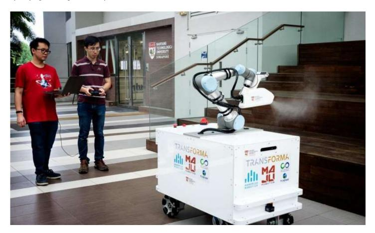
NTU's XDBOT can disinfect large surfaces quickly and can operate 4 hours continuously with its large disinfection tank and rechargeable batteries. Credit: NTU Singapore
