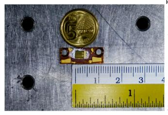
The electrically-driven topological laser prototype in the lab measures a tiny 4mm in length. A Singapore 5 cent coin was placed above it for size comparison. Credit: NTU Singapore
