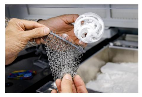
Examples of 3D printed products from the HP Multi Jet Fusion printer, which allows for flexible designs with both soft and hard plastic in a single print. Photo courtesy: HP Inc.
