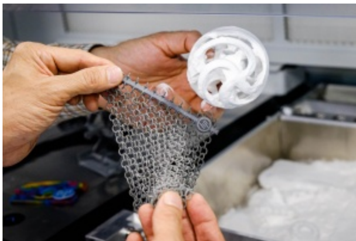
– Examples of 3D printed products from the HP Multi Jet Fusion printer, which allows for flexible designs with both soft and hard plastic in a single print
