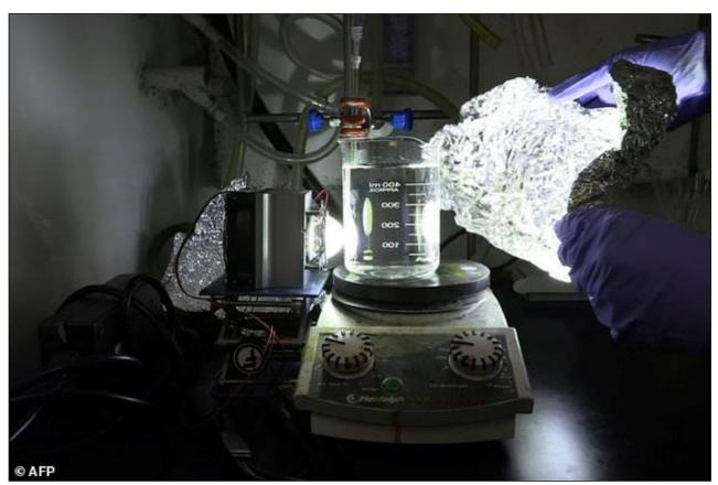
Plastic is mixed with chemicals into a solution which can be broken down by artificial sunlight, with scientists at Singapore's Nanyang Technological University hoping to replicate the process under real sunlight
