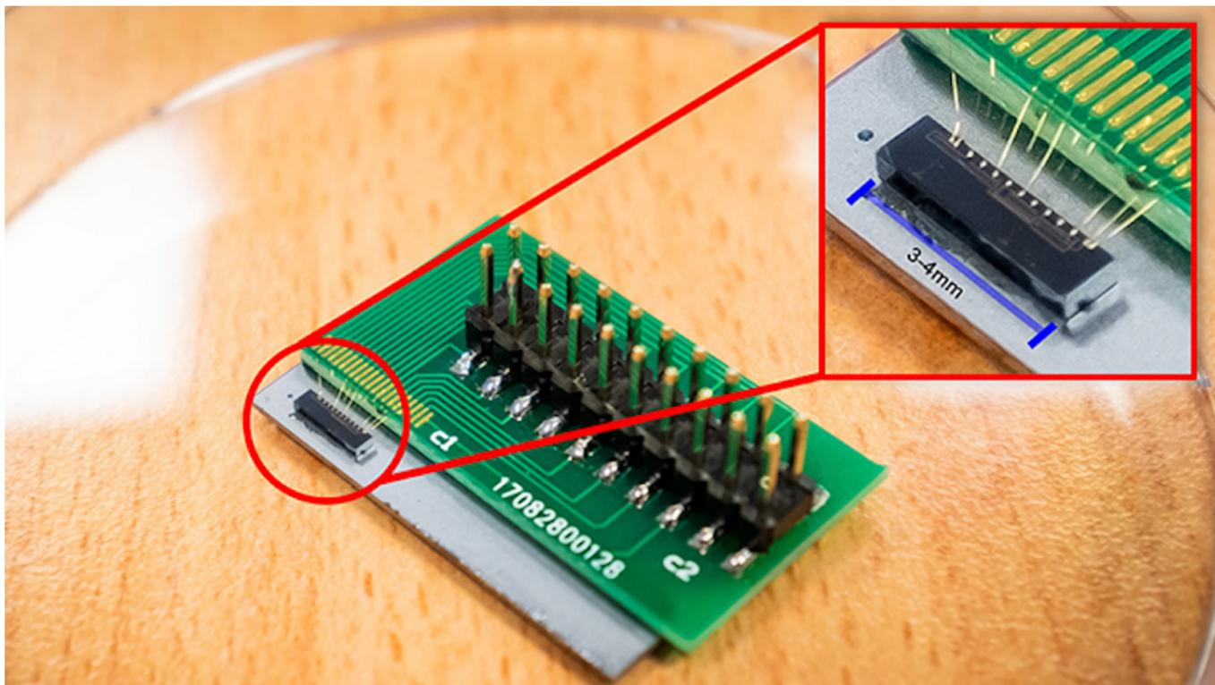
*Roughly about 3mm in size, the tiny chip developed by NTU scientists uses quantum communication algorithms to better security than existing industry standards. It also opens doors for more secure communication technologies that can be deployed in compact devices such as smartphones, tablets and wearables.*
