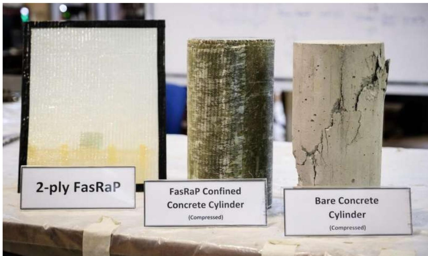
A 2-ply FasRaP hardened by light exposure, a concrete cylinder reinforced with FasRaP (middle) that can withstand twice as the load as the bare concrete cylinder which was cracked under high pressure (right). Credit: NTU Singapore
