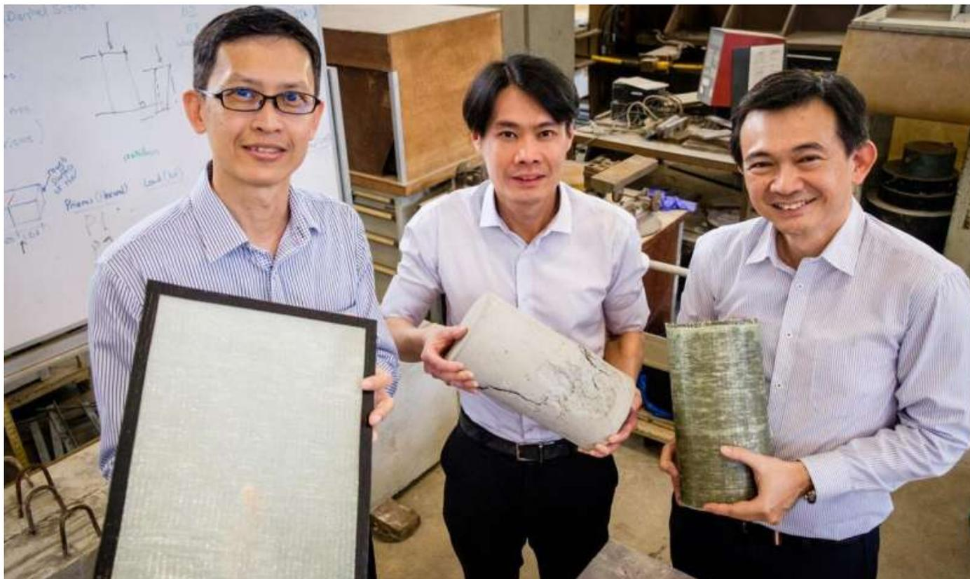
(from left) NTU Associate Professor Ng Kee Woei holding the FasRaP, JTC Group Director of Engineering Mr. Calvin Chung holding a concrete cylinder that was cracked under high pressure, and Prostruct Consulting Founder Dr. Ang Choon Keat holding a concrete cylinder reinforced with FasRaP, which can withstand twice the load compared to bare concrete. Credit: NTU Singapore
