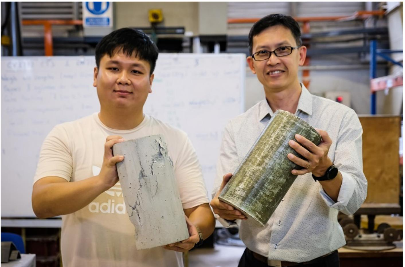
**FasRaP contains a proprietary glue-like resin which acts as an adhesive for the wrap developed by NTU materials scientists.** Nanyang Technological University
