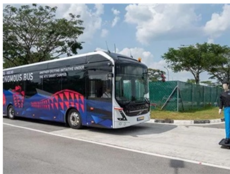
Volvo Buses and Nanyang Technological University (NTU) in Singapore have demonstrated the world's first 40-foot autonomous electric bus. Photo: Volvo
