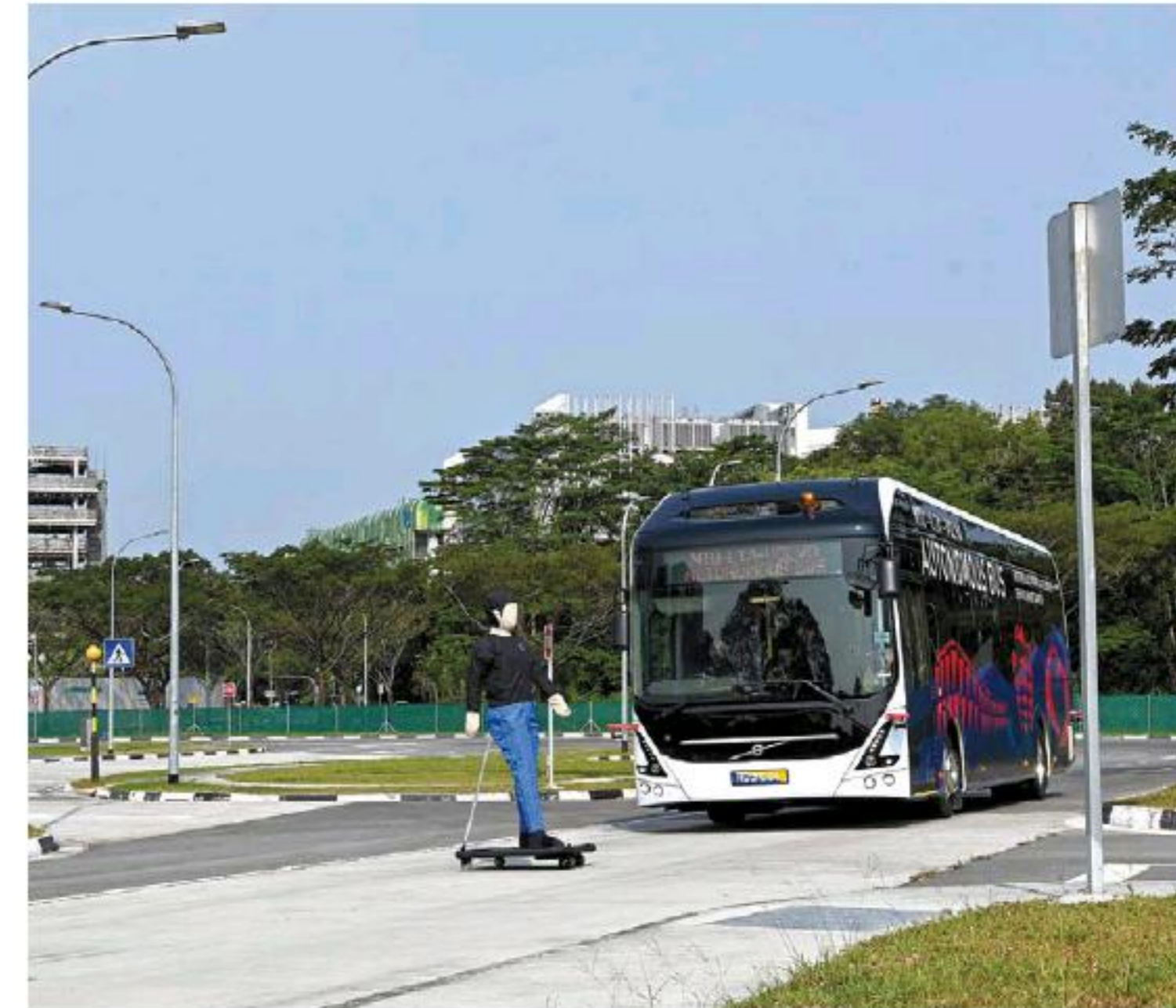
A Volvo AB 7300 electric autonomous bus drives on the track of Centre of Excellence for Testing & Research of Autonomous Vehicles. — AFP photo
