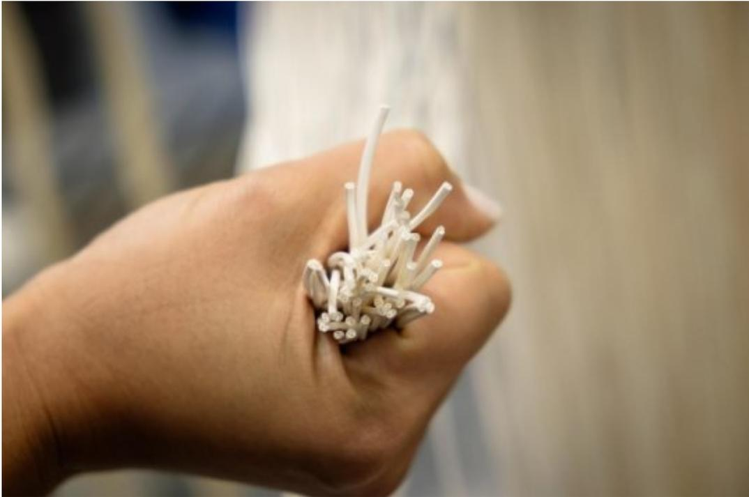
Close up shot of the tri-bore hollow-fiber membrane commercialized jointly by START Centre and Memsift Innovations, which will be used in a new pilot wastewater treatment plant for a semiconductor factory in Singapore.
