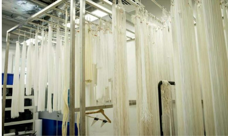
START Centre is a national-level facility in Singapore to develop and commercialise innovative separation and filtration technologies. This is a membrane production line at START Centre, which produces the tri-bore hollow-fibre membrane ... more
