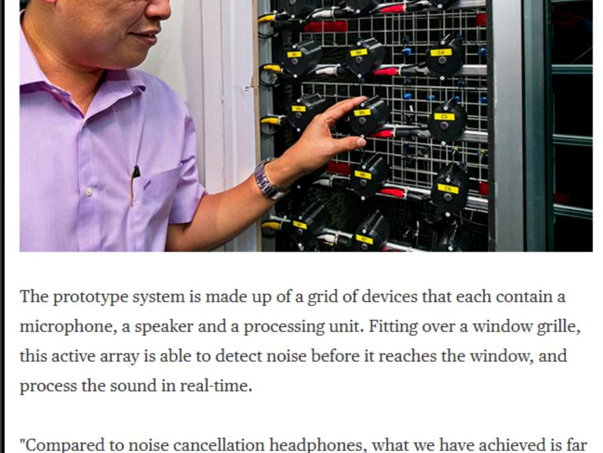
To test the system, the team built a replica room, complete with windows and doors, inside a soundproof chamber. The prototype was attached to the window, and to emulate outside noise, a speaker was set up to play recorded sounds like construction work and passing planes, trains and automobiles. The researchers say it managed to reduce the noise by up to 50 percent.
