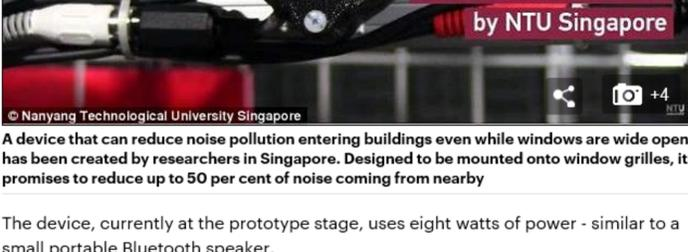
When both outside noise and anti-noise converge they cancel each other out, resulting in a softer ambient sound entering living spaces. Experts conducted tests on the technology using a soundproof chamber that houses a mock room with windows and doors
