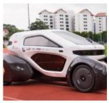
The NTU Venture (NV) 9 is a three-wheeled racing vehicle featuring hand-made silicon solar cells. According to Team Manager Winston Tan, inspiration for the vehicle originated in motorcycle racing, where riders lean to maintain handling and speed.
