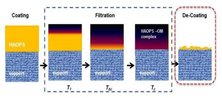
$T_c$  is a critical duration of the filtration at which the de-coating becomes imperative (as indicated by the higher pressure required to operate the subsequent treatment cycle).
