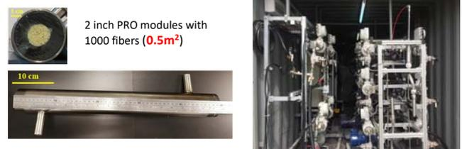
Fig. 4. Captures of pilot PRO modules (left) and pilot PRO test setup (right)
