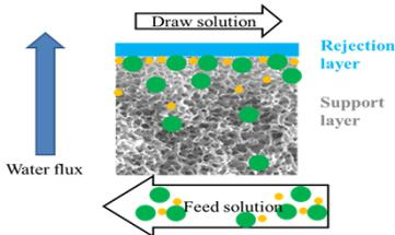
Fig. 2. Illustration of membrane fouling in PRO membranes.
