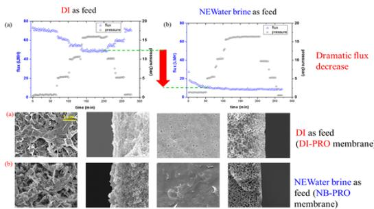
Fig. 5. PRO performance using DI water and NEWater brine as feed (up) and SEM images of the PRO membrane after test (down)
