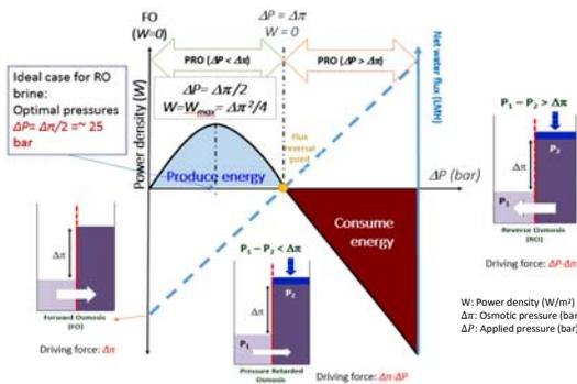
Fig. 1. Relationship of power density, net water flux and pressure in RO, FO and PRO process.
