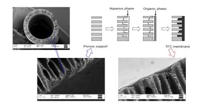
Approach 3: Layer-by-Layer (LBL) Deposition of Polyelectrolytes
