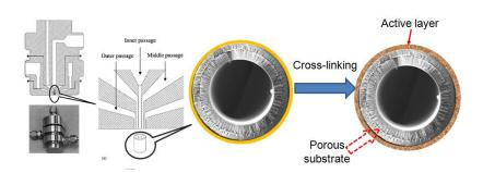
Approach 2: Thin Film Composite membrane by in-situ interfacial polymerization (IP)
