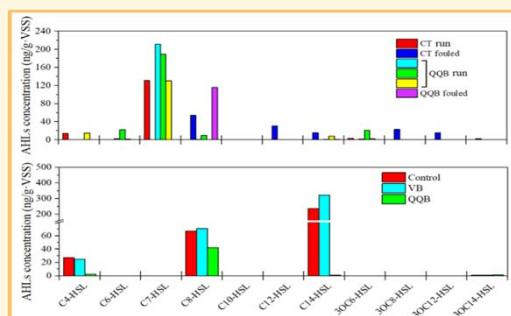
AHL concentration in biocake declined in QQ reactor compared to control reactors
