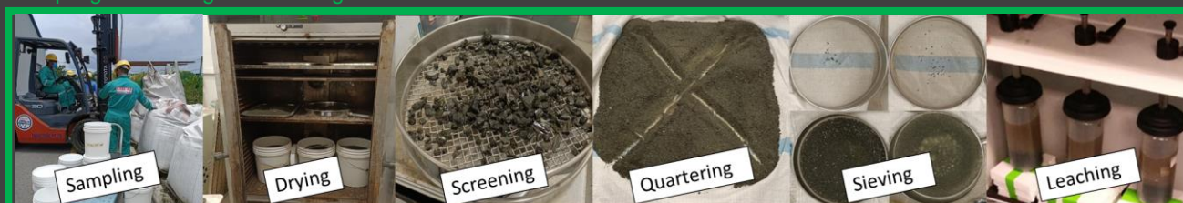
Sampling and testing of MSW slag
