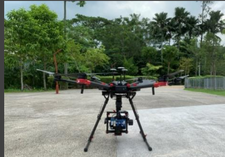
EPMC's hyperspectral UAV system
