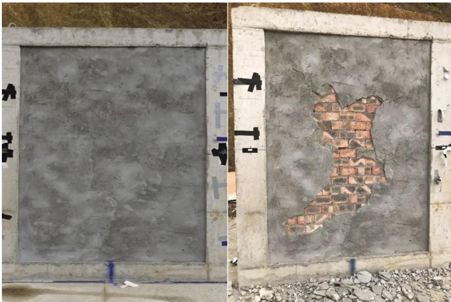
A wall wrapped with the material (left). It was left largely undamaged despite a luggage bomb exploding around 10 metres away. PHOTO: NANYANG TECHNOLOGICAL UNIVERSITY
