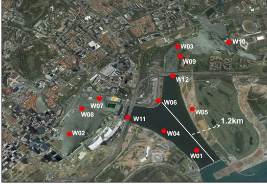
Figure 1: Locations of deployed wind sensors on and around an urban reservoir in Singapore.
