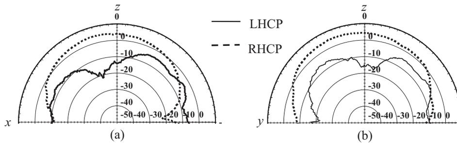
**Figure 4** Radiation pattern of the proposed antenna at 3740 MHz. (a)  $x$ - $z$  plane (b)  $y$ - $z$  plane
