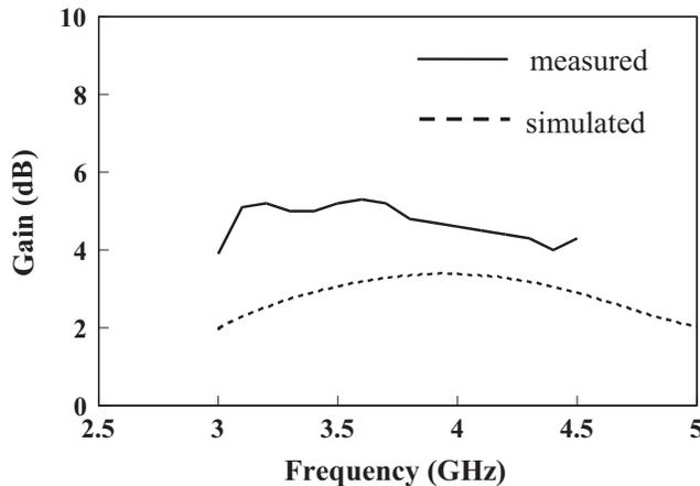
**Figure 5** Gain variation against frequency for proposed antenna plane (b)  $y$ - $z$  plane
