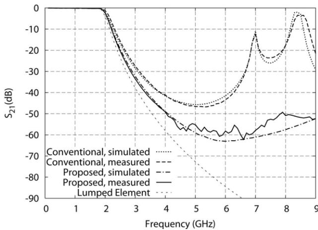
**Figure 3** The simulated and measured  $S_{21}$ -parameters of the proposed and the conventional stepped-impedance low-pass filter, and the simulated  $S_{21}$ -parameter of their corresponding circuit model
