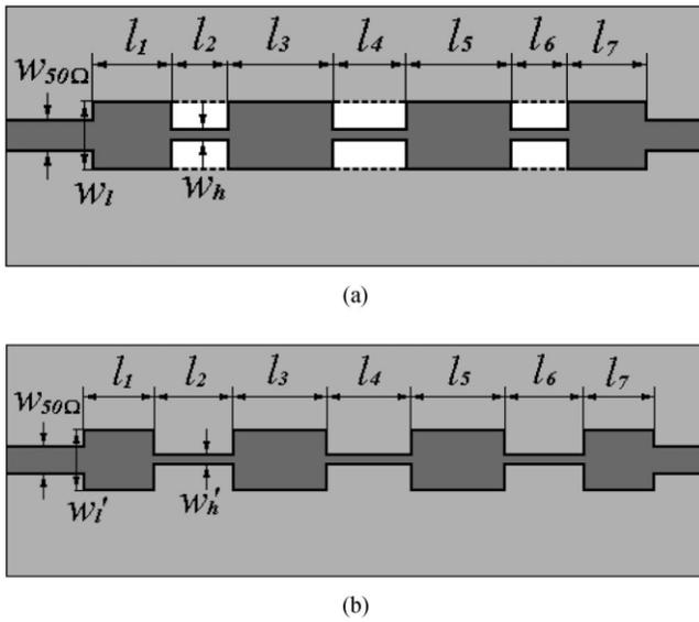
**Figure 2** (a) The schematic of the proposed stepped-impedance low-pass filters with slot-back microstrip line sections. (b) The schematic of the conventional stepped-impedance low-pass filter
