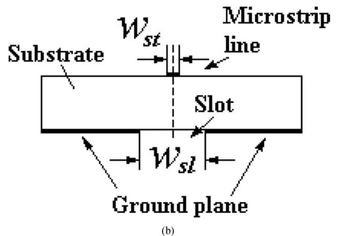
**Figure 1** (a) The top view of a slot-back microstrip line. (b) The cross-sectional view of a slot-back microstrip line
