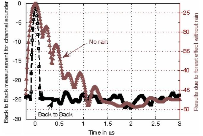
Fig. 2. Power delay profile for back-to-back measurement and forested propagation without rain effect.
