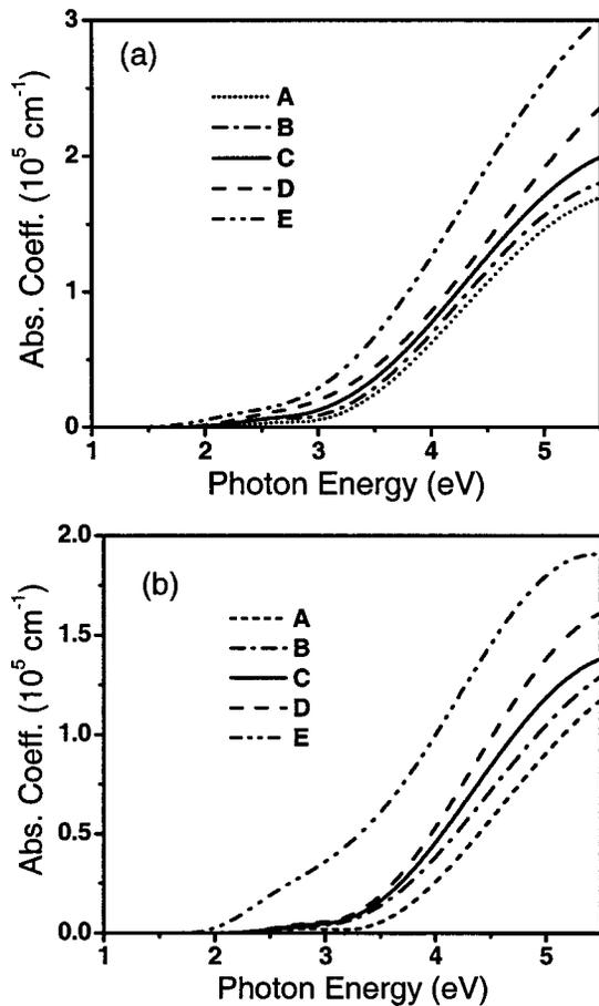
FIG. 4. Comparison of room temperature absorption spectra of (a) as-grown Ref. 4 and (b) fluorinated *p*-Si samples, from which the PA energies are derived with the Tauc plot method.
