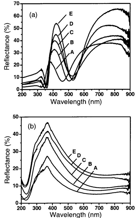
FIG. 3. Room temperature reflection spectra of (a) as-grown and (b) fluorinated  $p$ -Si samples.
