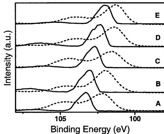
FIG. 5. Size-dependent XPS Si- $2p$  profiles of as-grown (dash line) and fluorinated (solid line) *p*-Si samples.
