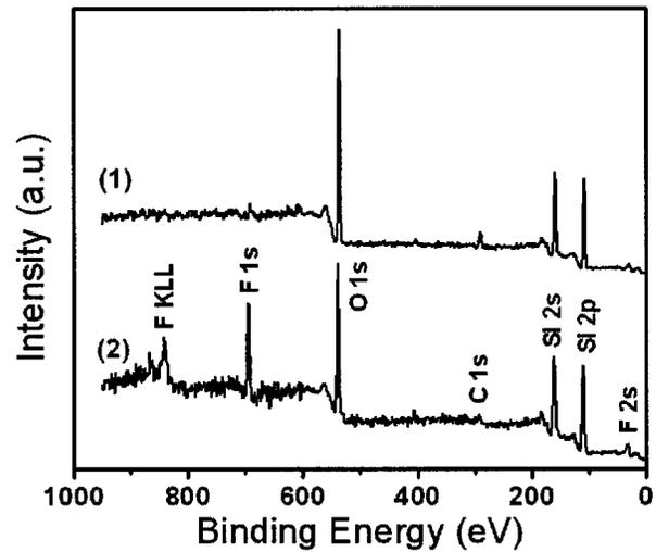
FIG. 1. XPS spectra of the  $p$ -Si sample  $E$  before (1) and after (2) fluorination. It shows the existence of fluorine in fluorinated sample.
