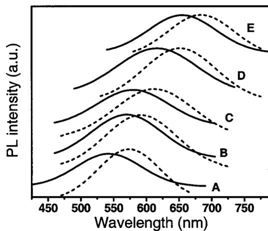
FIG. 2. Size-dependent PL spectra of as-grown (dash line) and fluorinated (solid line)  $p$ -Si samples. The data of sizes are given in Table I.
