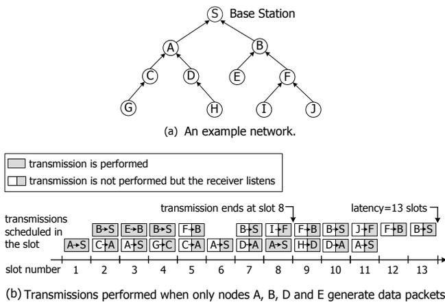
Fig. 1. Inefficiency of a schedule targeted on a static network traffic pattern.
