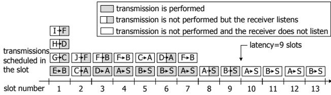
Fig. 3. The TPO schedule constructed for the network of Fig. 1(a).
