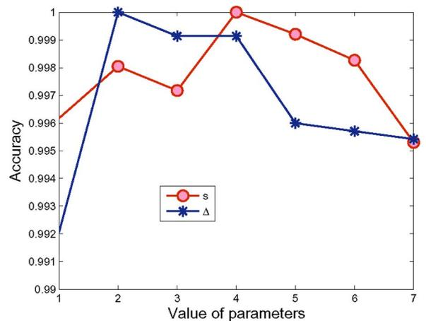
Fig. 7. Sensitivity of parameters on the performance of cluster separation: the diameter of the structuring element  $s$  and tolerance value of the adaptive threshold  $\Delta$  (in pixel values).
