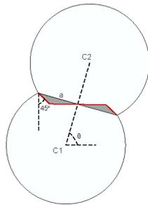
Fig. 4. Shaded triangles show the errors due to jagged lines created by classical watershed algorithm using inner distance map as the marking function.
