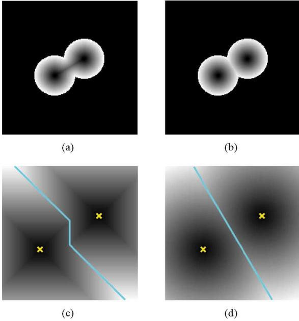
Fig. 2. Euclidean distance map using (a) inner distance transform and (b) outer distance transform. The distance map of two pixels, created by (c) the chessboard distance and (d) the Euclidean distance.
