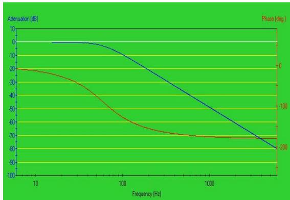
Figure8 Frequency response of the 2nd order low pass filter
