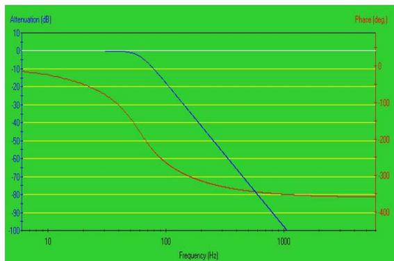
Figure9 Frequency response of the 4th order low pass filter
