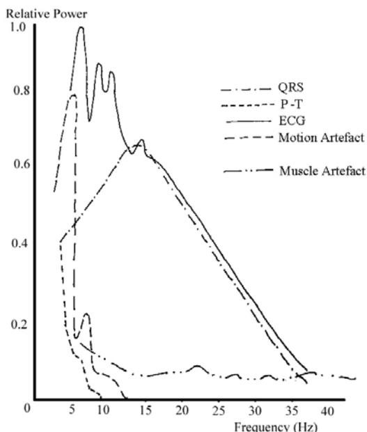
Figure4 Power spectra density of ECG
