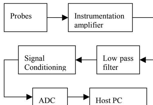
Figure5 Basic Framework of the PC based ECG monitoring system
