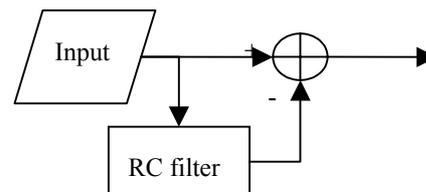
Figure 10 Block diagram of prototype DC offset remover
