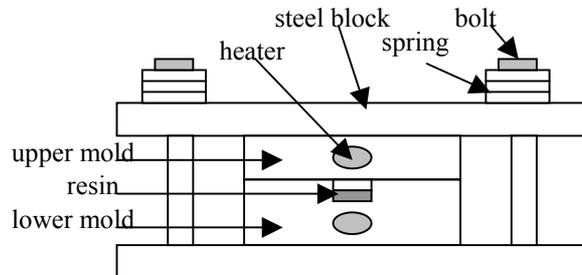
Fig. 2: Schematic of compression molding apparatus
