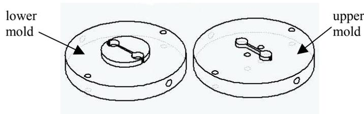
Fig. 1: Stainless steel mold
