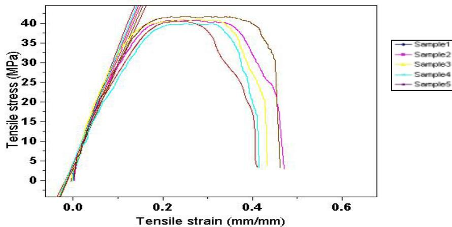
Fig. 7: Stress-strain graph for composite
