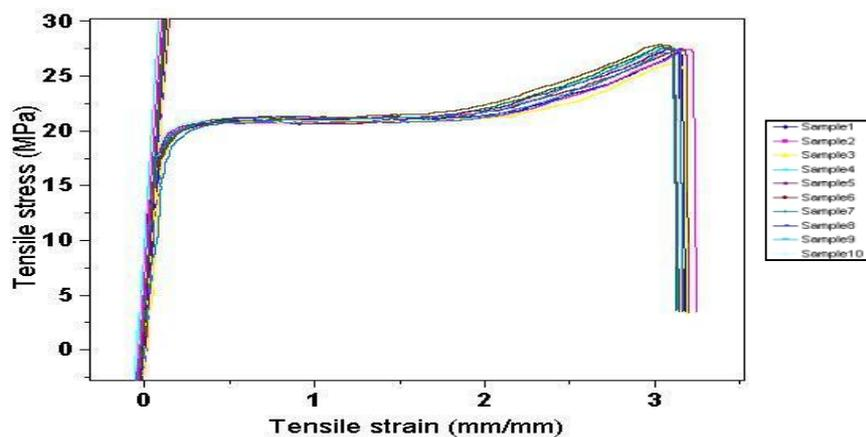
Fig. 6: Stress-strain graph for UHMWPE
