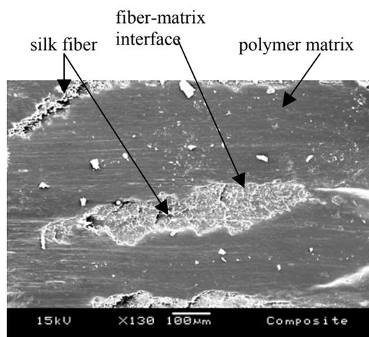
Fig. 8: Composite cross-section x130 magnification
