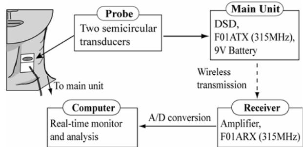
**Figure 1:** Portable measurement system of blood flow velocity with real-time monitoring.
