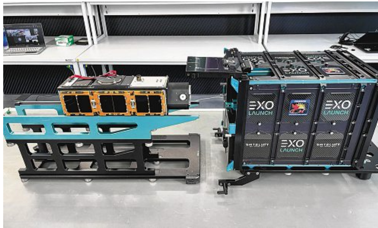
The CRIMSON-1 satellite (left) being integrated into the EXOpod Nova system, which deployed the satellite into space after it was launched. PHOTOS: NTU
