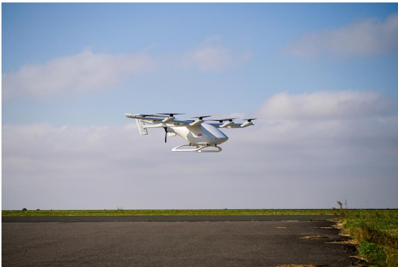
Image: The 8-metre wingspan eVTOL prototype taking flight at DLR.
