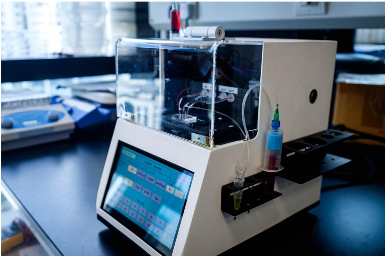
Prototype of the ExoArc system, which allows for a one-step automated isolation of high-quality blood plasma useful for diagnostics and precision medicine.
