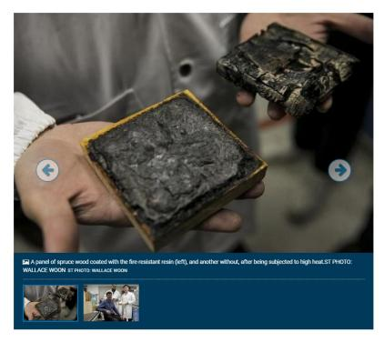
One crackled and blackened, as expected, and the other started foaming up, with its surface expanding to form a layer of insulation, protecting the wood underneath.
