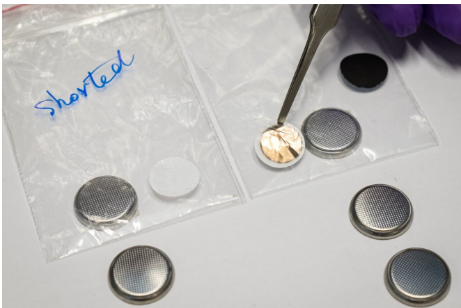
The NTU anti-short layer (upper right held by tweezers) stops short circuits from happening in li-ion batteries. Credit: NTU Singapore
