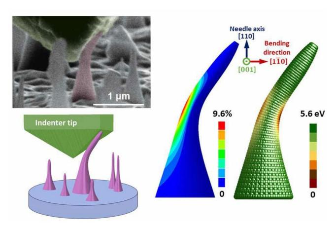
Tiny needles of diamond are strained by bending, as seen in electron microscope image, top left. Computer simulations show the effects, with normal insulating properties in green, and areas with metallic properties, never seen before in diamond, in deep red. Courtesy: Massachusetts Institute of Technology (MIT)
