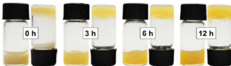
Image 3: Pollen at different incubation times. As incubation time increased, the pollen developed a greater degree of gel-like characteristics, as indicated by decreased resistance to flow under the influence of gravity.
