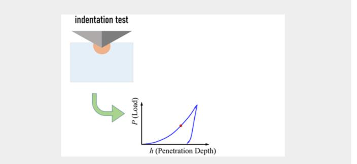
Animation showing schematically the process of extracting mechanical properties from indentation tests. It is a challenging task to accurately obtain the yield strength and nonlinear mechanical behavior from indention tests. Illustration by the researchers.
