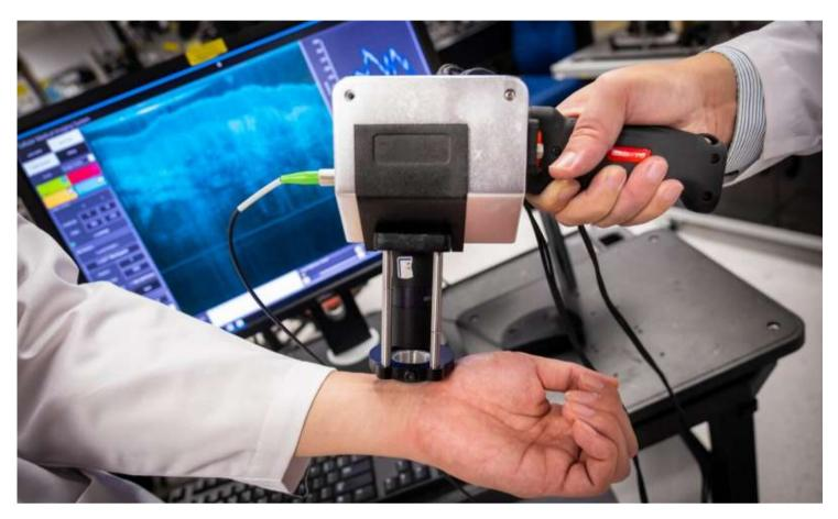
The prototype handheld medical imaging device developed by NTU Assoc Prof Liu Linbo can produce high-resolution images in real-time, and was also designed to be used by medical professionals who do not specialise in imaging or pathology, allowing them to scan patients using the new device in community clinics or at the bedside. Credit: Nanyang Technological University
