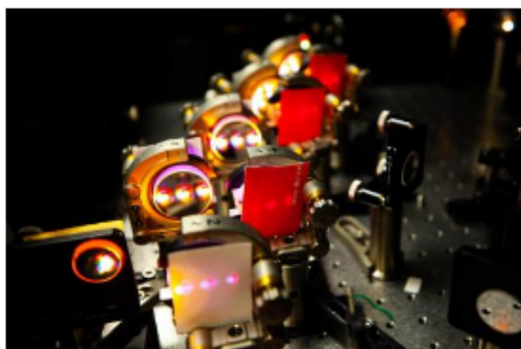
IMAGE: The comprehensive setup that Assoc Prof Loh from NTU Singapore used, which includes a chirped mirror compressor to generate 5-femtosecond laser pulses. This allows for the observation of radiation damage...
