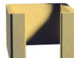
**3** Bathroom unit printed in nine hours. The first part was printed in six hours and the top part in three hours (the structure has to be printed in two parts due to space constraint in the lab)
