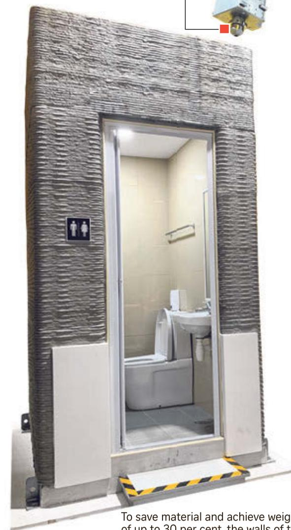
To save material and achieve weight savings of up to 30 per cent, the walls of the prefabricated bathroom are printed in a W-lattice shape, which lends additional strength to the final structure.
