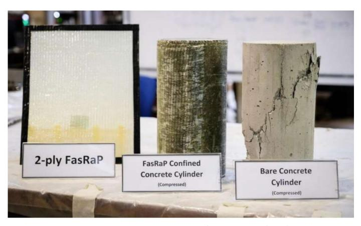
A 2-ply FasRaP hardened by light exposure, a concrete cylinder reinforced with FasRaP (middle) that can withstand twice as the load as the bare concrete cylinder which was cracked under high pressure (right). Credit: NTU Singapore
