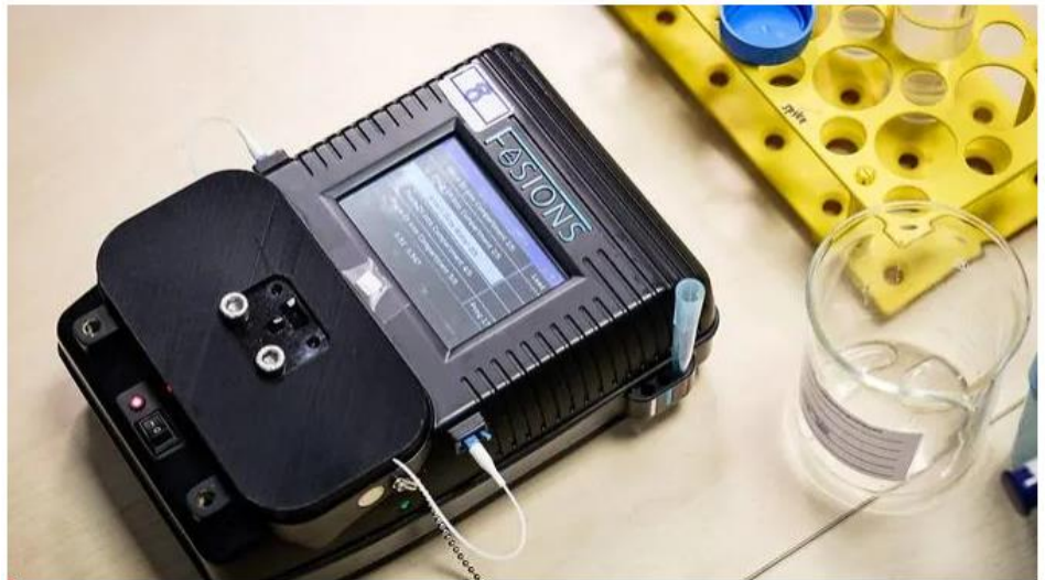
The device generates test results quickly without the need to bring samples back to laboratories, facilitating on-site water testing. (Photo: NTU Singapore)
