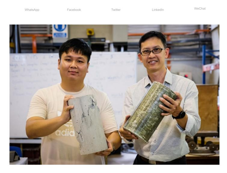
FasRaP contains a proprietary glue-like resin which acts as an adhesive for the wrap developed by NTU materials scientists. Nanyang Technological University
