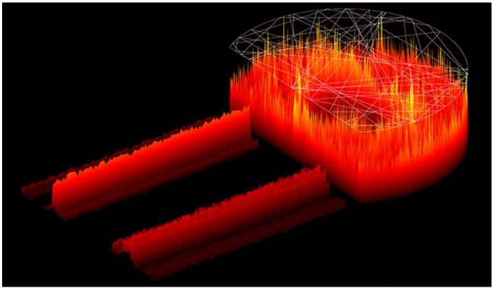
D-shaped laser cavity tackles instability in high-powered lasers (Credit: Yale University)
