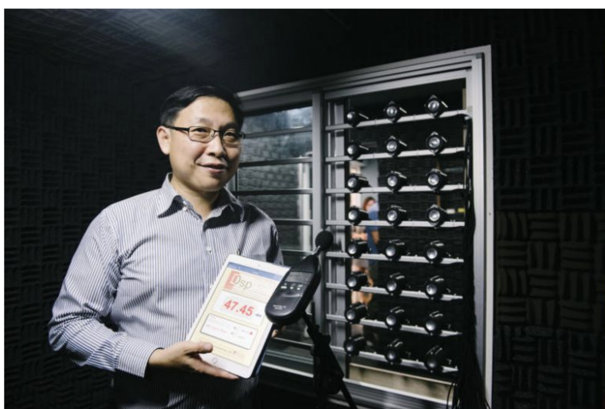
Professor Gan Woon Seng of NTU, lead researcher of the team that developed a device that can reduce noise pollution entering buildings even while windows are wide open. ST PHOTO: ALVIN HO
