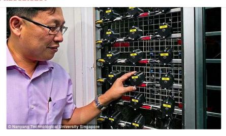
Several units are placed together to form a grid-like array on a window grille to reduce external noise by emitting 'anti-noise' signals. Researchers are working to further improve the technology's efficiency, making them smaller, more cost-effective to produce
