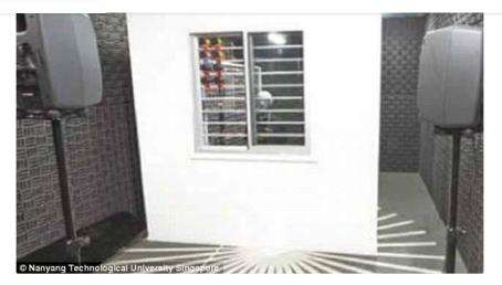
When both outside noise and anti-noise converge they cancel each other out, resulting in a softer ambient sound entering living spaces. Experts conducted tests on the technology using a soundproof chamber that houses a mock room with windows and doors
