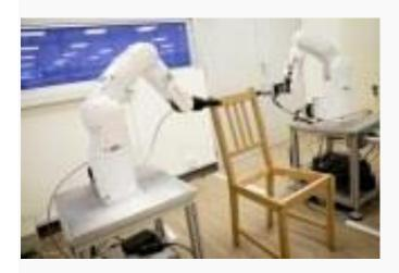
Each robotic arm is equipped with parallel grippers to pick up objects and has force sensors to determine how strongly the "fingers" are gripping.
