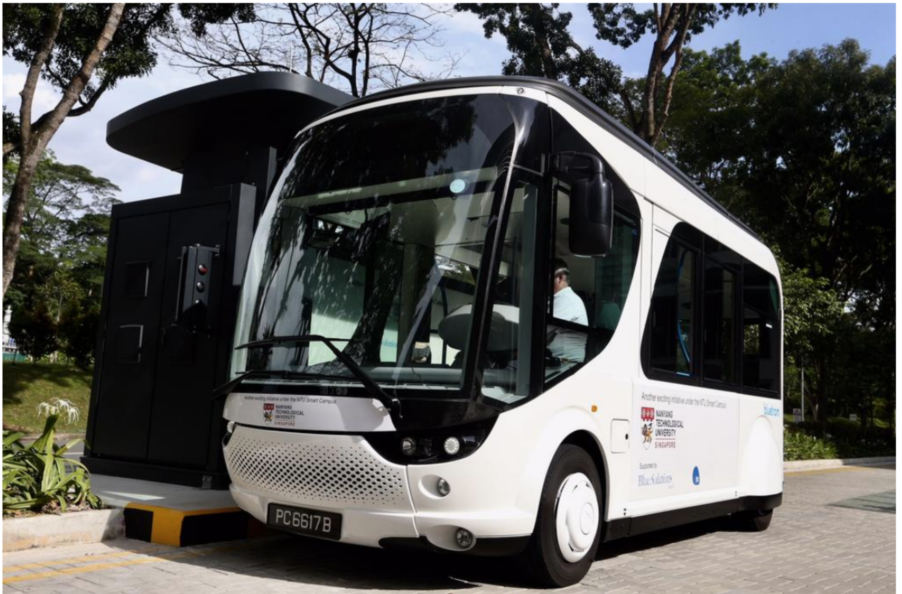
The shuttle can travel two kilometres on a single charge, with backup power that can allow it to run for an additional 30 kilometres. Photo: Koh Mui Fong/TODAY
